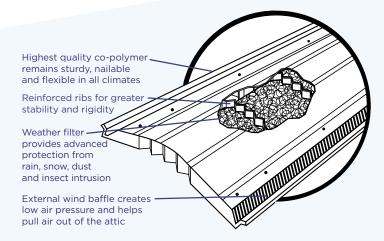
Meets UL manufacturing quality standards and code requirements for Class A fire-rated roof decks
